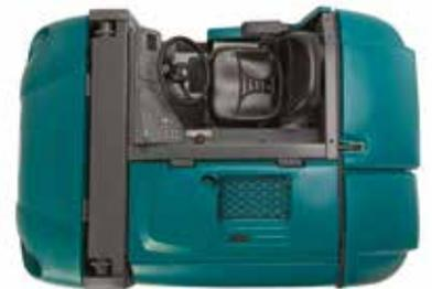
Achieve outstanding results in diverse environments with dual side brushes which, combined with a large 395 L Duramer™ hopper, allow you to sweep up to a path width of 2030 mm in a single pass.
